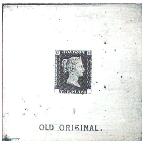
The original recess metal die for the Penny Black, engraved in reverse, without corner letters
